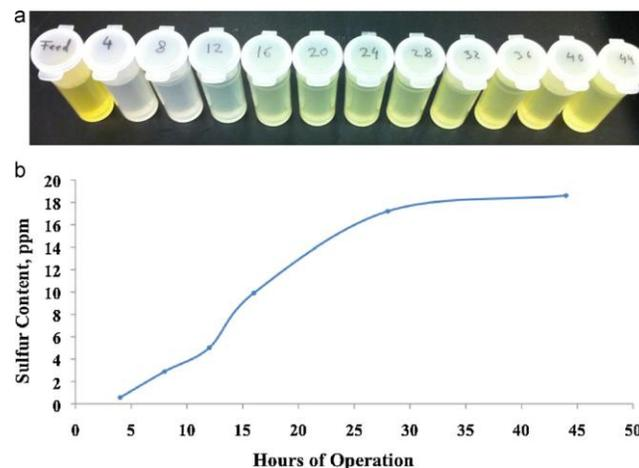
Figure 1. Desulfurization test results: (a) photographs of diesel samples taken at various times on stream; and (b) the quantification of sulfur content in the treated diesel.
