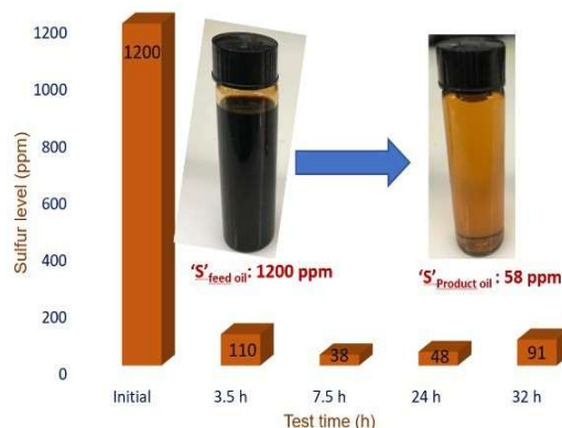
Desulfurization of used motor oil (UMO) AdE-Sulfur™-010 at atmospheric pressure
